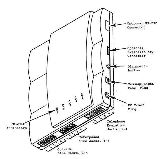
To understand how the Classic Mail operates it is important to understand the concept of Telephone Emulation and Interposed lines.
